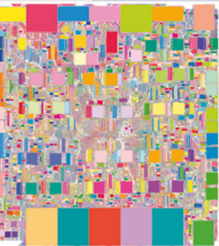
Picture: A placement of a system controller which was computed with the BonnTools.
